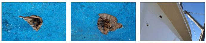
With some expert shipwright assistance, the holes below the waterline have been repaired, and a new coat of antifoul applied.
